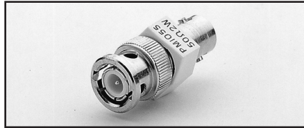
Model 7755 50Ω Feed-Through Terminator: BNC-to-BNC adapter for terminating RG58 cable in its characteristic impedance. VSWR < 1.1, DC-250MHz.
